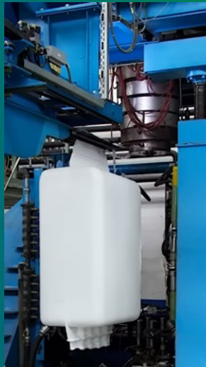
Blow molding system
