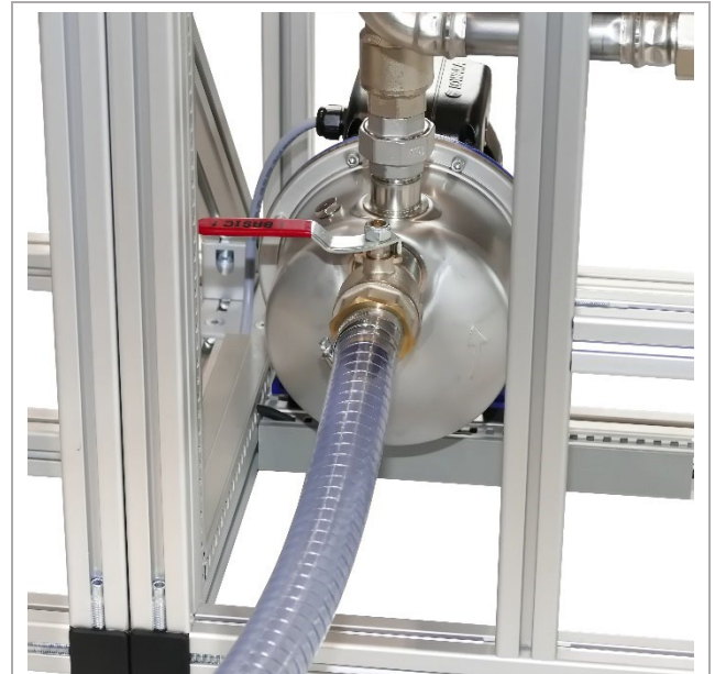
Figure 10: Attach the 1 ¼ inch (GWtec® 140/240) and 1 ½ inch (GWtec® 340/440/640) PVC hose to the filtrate pump using the (three-part) brass pipe union.
