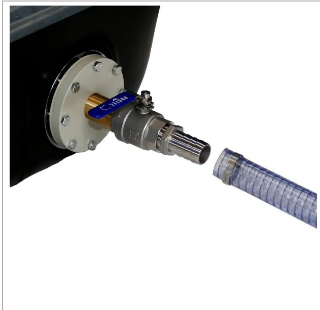
Figure 9: Attach the 1 ¼ inch (GWtec® 140/240) and 1 ½ inch (GWtec® 340/440/640) PVC hose to the greywater filtration tank using a stainless-steel hose clamp.
